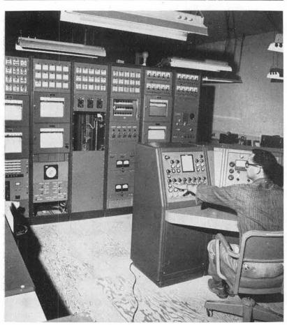
CONTROL CONSOLE for new reactor is operated here by Norman Lucas (5431). The instrumentation is a combination of commercial and Sandia-designed parts. Missing panel in center of photograph is at reactor site to check out the cooling system.
